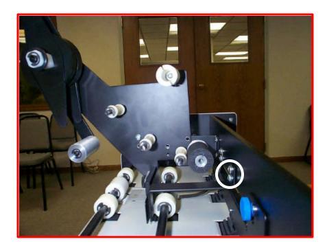
When running some translucent tabs, it may be necessary to decrease the amount of distance between the tab sensor and the peel bar.
